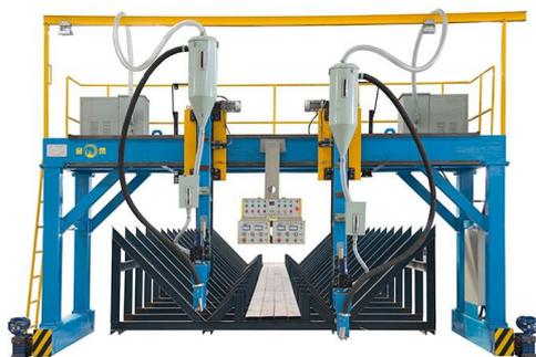
JINFENG WELDCUT is a professional China manufacturer and supplier of H beam welding machines with affordable price. The H beam welding machines are high performance machines to execute the submerged arc welding on full length of the H beam. It can do single arc or tandem arc welding as per the needed of customers.
