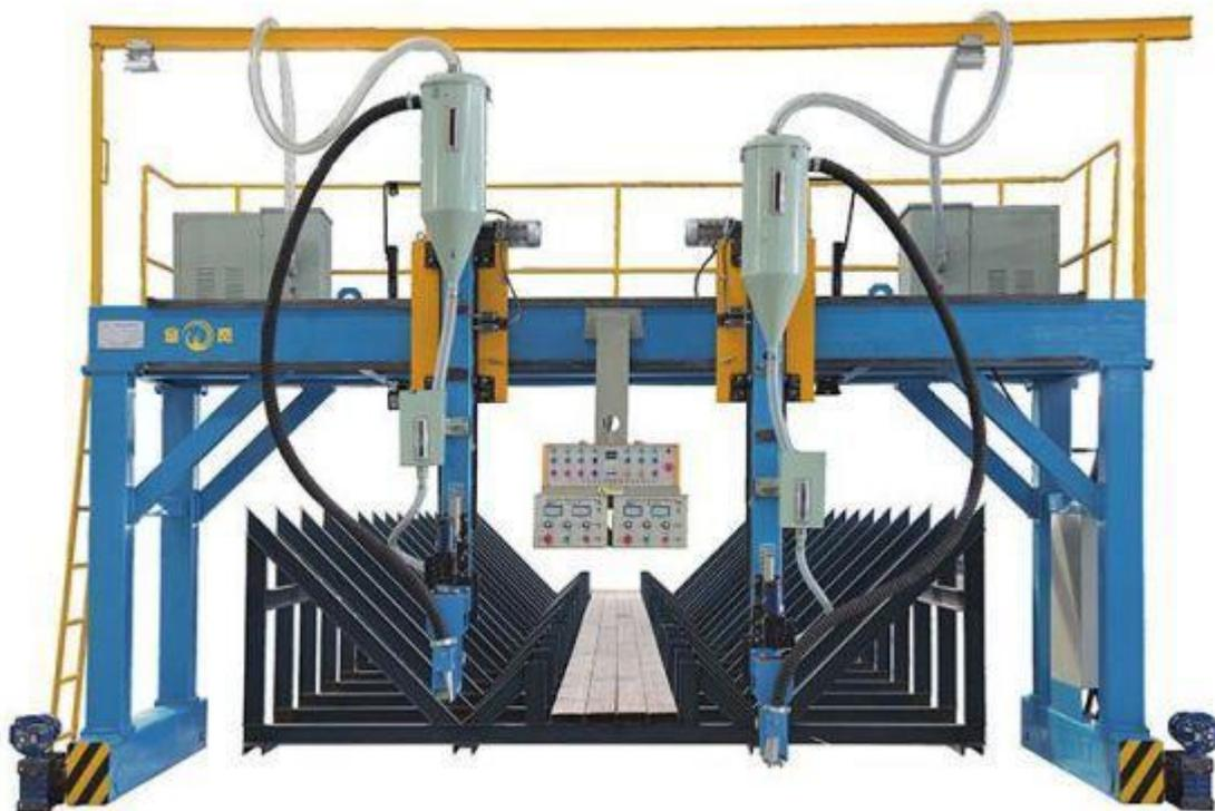
**H beam welding machines** in Gantry type MZG
