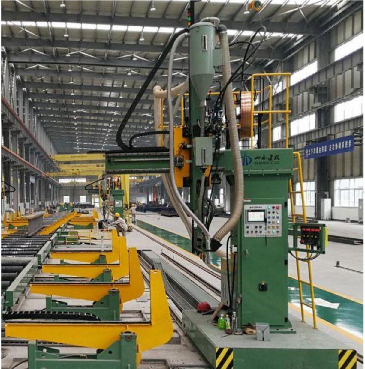
**H beam welding machines** in T Cantilever type TMH14
