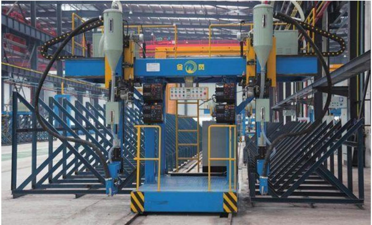
**H beam welding machines** in T type TMH14
